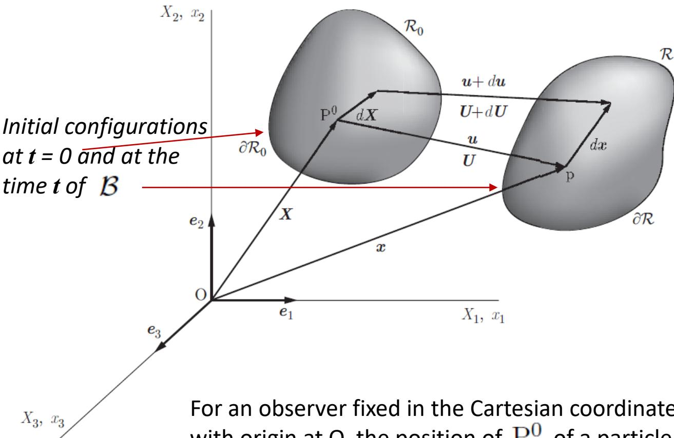
For an observer fixed in the Cartesian coordinate system with origin at  $O$ , the position of  $P^0$  of a particle of  $\mathcal{B}$  at  $t=0$  is represented by its **initial position** vector  $X$  and its **current position**  $p$  at time  $t > 0$  by the current position vector  $x$ .
