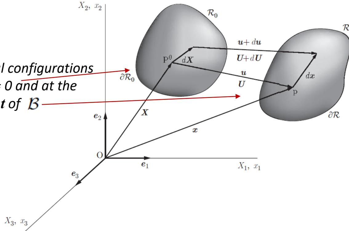
A particle is initially ( $t = 0$ ) at  $X$  and after a time  $t$  is at position  $x$ .
