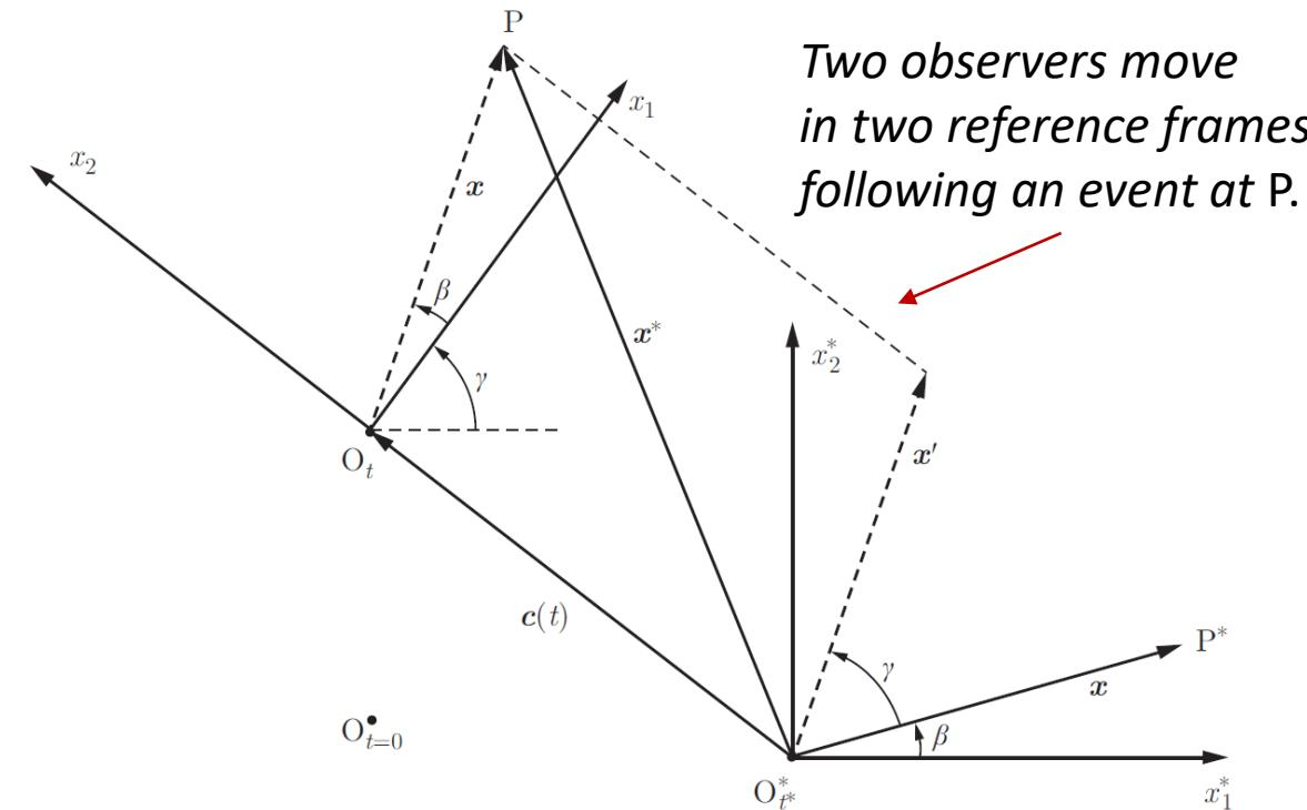
The same observation at P (experiment) seen by two observers in the corresponding reference frames at the same time. For the observer at  $R$  the vector position is  $x$ . For the observer at  $R^*$  we must take into account the rotation of  $R$  with respect to  $R^*$ .
